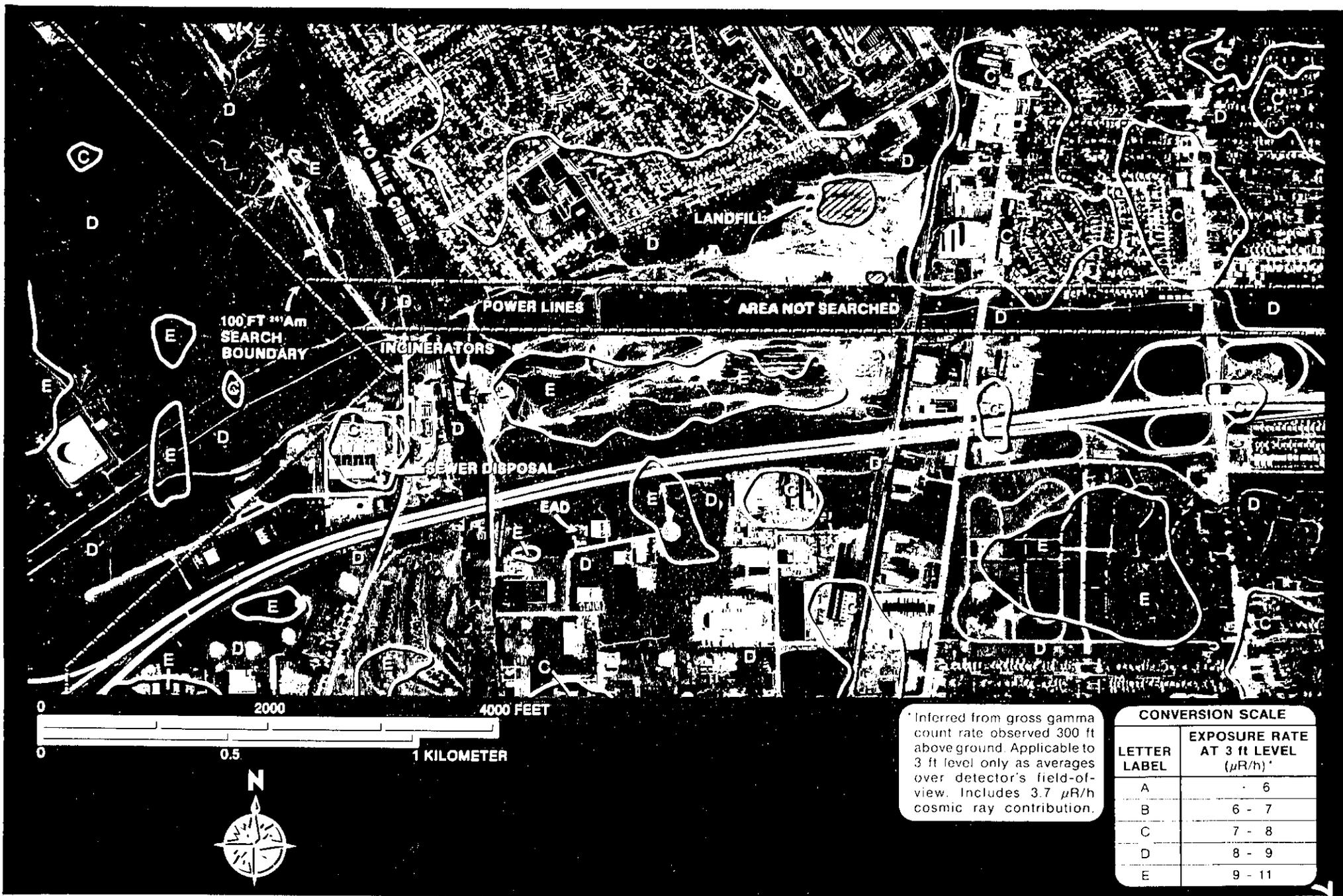
Figure 2. CLOSE-UP VIEW OF THE AERIAL RADIOLOGICAL SURVEY AND SEARCH RESULTS IN THE AREA OF PRIMARY INTEREST. Blue cross-hatching denotes <sup>241</sup>Am contamination.
