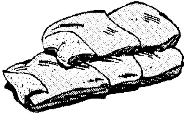
Stagger the joint connections when multiple layers are necessary. For unsupported layers over three courses high, use the pyramid placement method.
