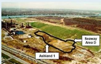
**Remediation of the Ashland 1 Site (and the Seaway D site) began in June 1999 and was completed in December 2002. 172,900 tons removed and disposed of out-of-state**
