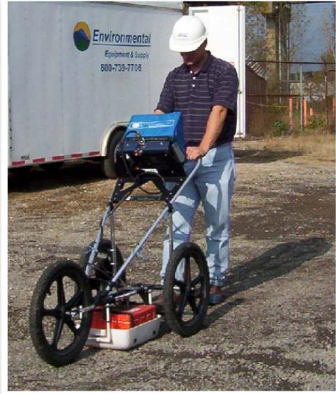
Subsurface investigation being performed using specialized radar equipment.
