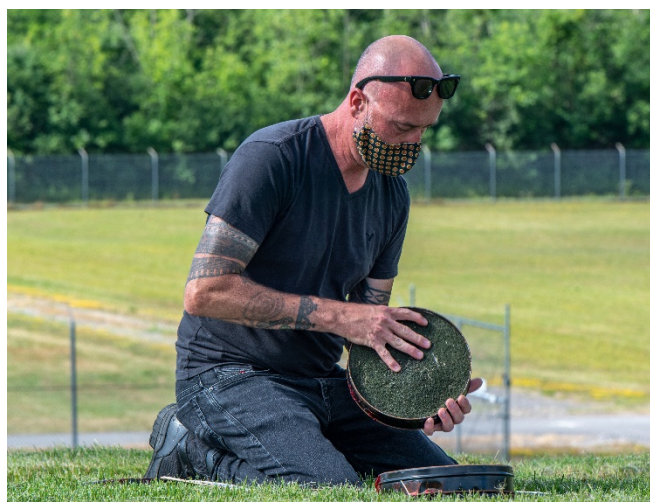
Figure 2: Activated charcoal canister being placed on the IWCS to measure radon flux
