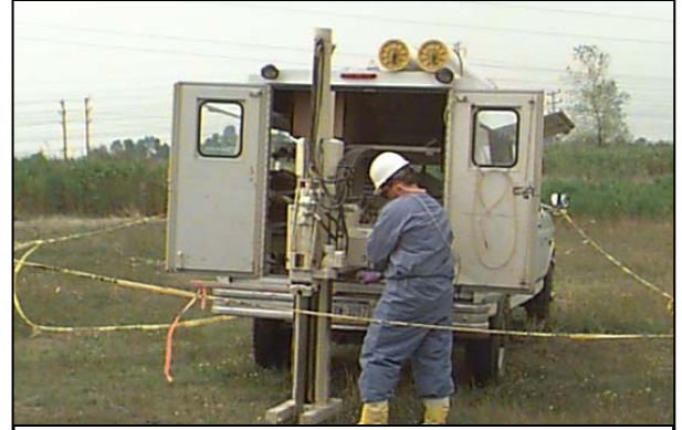
Collecting a subsurface soil sample at the Tonawanda Landfill in 2001
