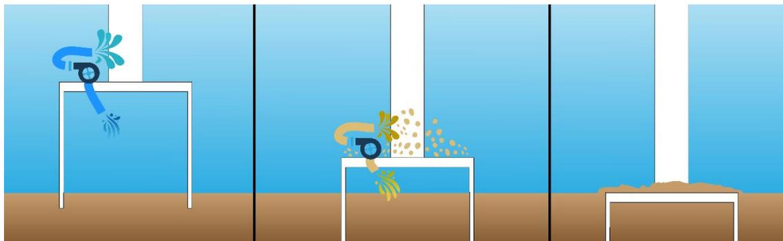
Inset 1. Sediment Deposition on to MB Foundation Lid
